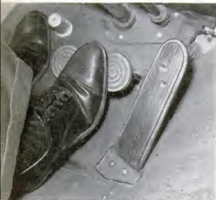
Brake and clutch pedals are too small, too crowded, says Clymer. That is the modified accelerator pedal
